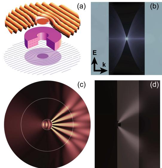
Transformation optics devices: a): cloak, b): light concentrator, c): impedance-matched hyperlens, and d): planar hyperlens
